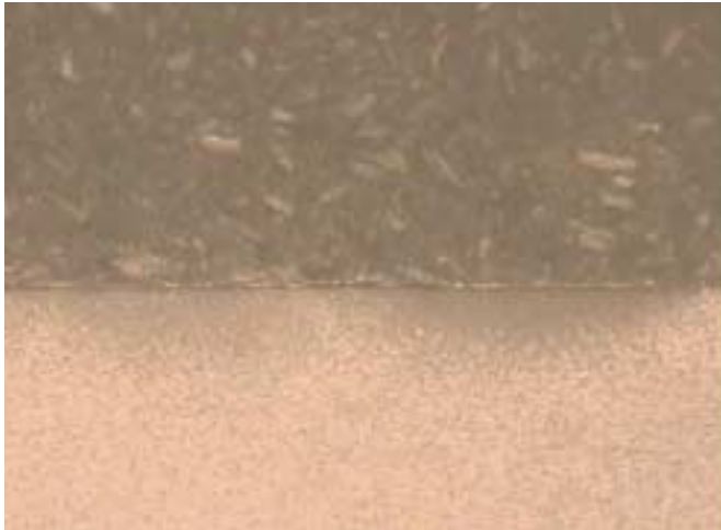
Fig 4 Photomicrograph of a cross section of a hardened zone in an SAE 1117 shaft. Maximum hardness is 47 HRC, with a hardness 41 HRC at a 0.5 mm (0.02 in.) case depth.
