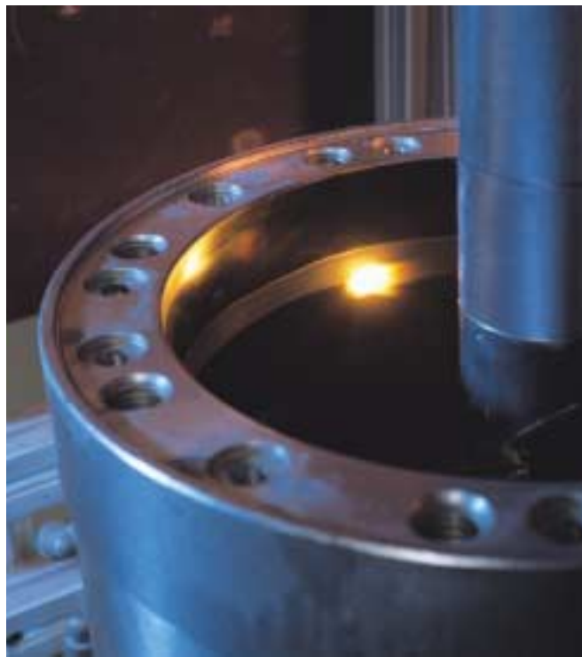
Laser heat treating of a cast iron cylinder
