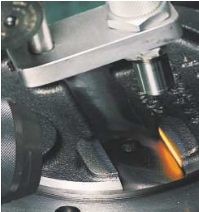
Specific localized area laser heat treatment of gray iron casting to 50 HRC at 1 mm (0.04 in.) depth
