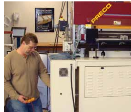
Service technician Robert Biggler performing a preventive maintenance voltage check.
